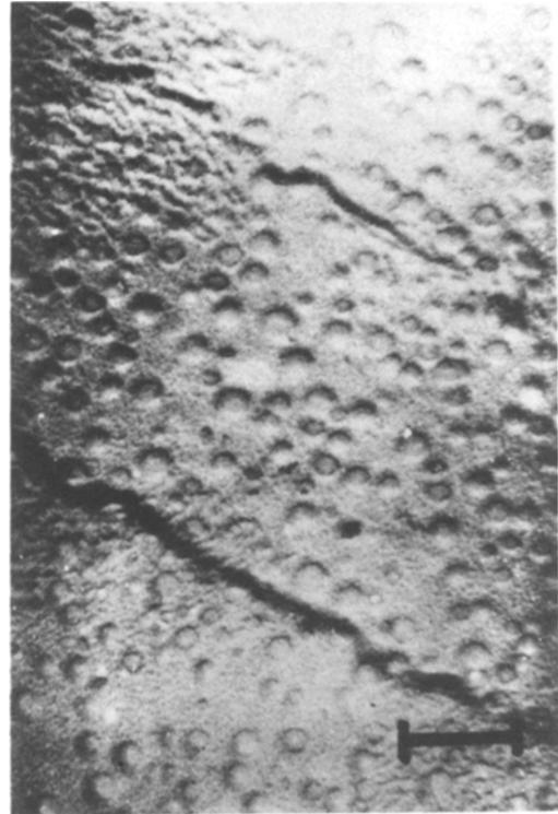
Figure 1 Fracture surface of 10PbO·90B<sub>2</sub>O<sub>3</sub> (wt %) sample, showing PbO-rich particles in a B<sub>2</sub>O<sub>3</sub>-rich matrix. Bar indicates 1  $\mu\text{m}$ .
